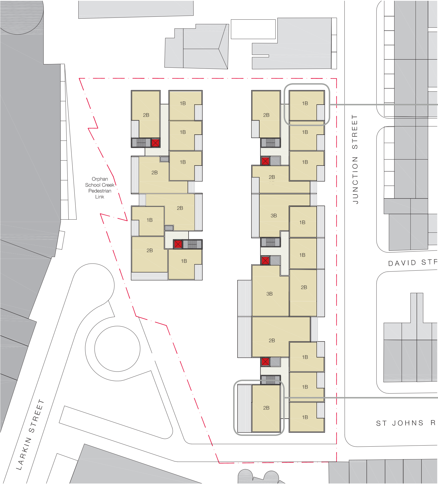
INDICATIVE PLAN - TYPICAL 1 BED plan can be oriented towards Junction street to maximise outlook and avoid overlooking issues. Translucent or screened glazing can provide cross ventilation and ventilation to kitchen
