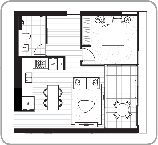
INDICATIVE PLAN - TYPICAL 1 BED plan can be oriented towards Junction street to maximise outlook and avoid overlooking issues. Translucent or screened glazing can provide cross ventilation and ventilation to kitchen
